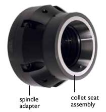
Check the concentricity and face runout of the spindle adapter before mounting the collet seat assembly. Neither should exceed .0002" ( $5\mu m$ ). If the indicator reading is more than .0002" ( $5\mu m$ ), remove the spindle adapter and clean the surfaces again before remounting.
